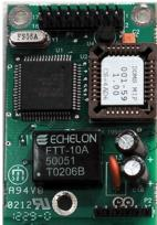
This module supports "free topology", which means that the LON interface can be connected directly to a number of devices without point to point terminations. Alternatively, the module can be supplied with a LON-connector
