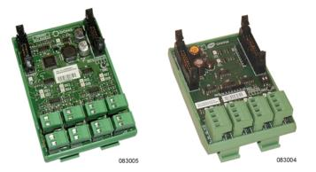
**Note:** The black serial connectors on the DMB modules are wider than those on the DSB models. This extra width is a result of more pins, which are required for the signals used to control the onboard multiplexer.
